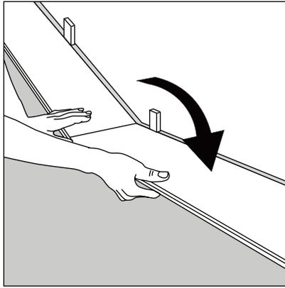
② Begin laying in the left-hand corner. Place the plank 1/2" (10mm) from the left wall with the tongue side of the plank facing the wall. Use spacers between the wall and the plank.
