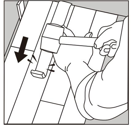
③ First row, last plank: At the end of the first row, leave an expansion gap of 1/2" (10mm) to the wall and measure the length of the last plank to fit. Insert the short side and tap it closed, using a pull bar.
