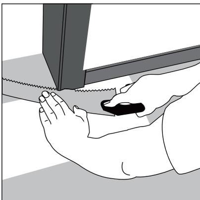
**10** Door molding and skirting: lay a board (with the decorative side down) next to the door molding and as shown in the figure. Then slide the floorboard under molding.
