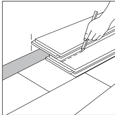
**8** To lay the last row: position a loose board exactly on top of the last row installed. Place another board on top, with the tongue side touching the wall. Draw a line along the edge of this boards, to mark the first board. Cut along this line to obtain the required width. Install the long side tongue into the groove with the end joint aligned. Using a pull bar and hammer, work evenly along the length of the plank and lightly tap the joint closed.
