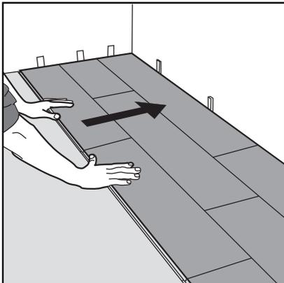
**7** After 2-3 rows. Adjust the distance to the front wall by leaving an expansion gap of 1/2" (10mm). Always ensure that the end joints are staggered at least 12" (30cm) from one row to the next.
